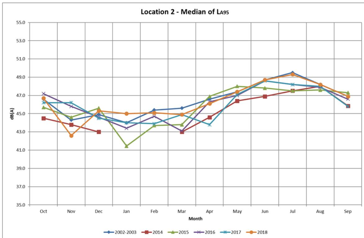
**Figure 6-3 Comparison of noise levels measured at Location 2 (South Monitor) for base period (2002 – 2003) and 2014 – 2018**
