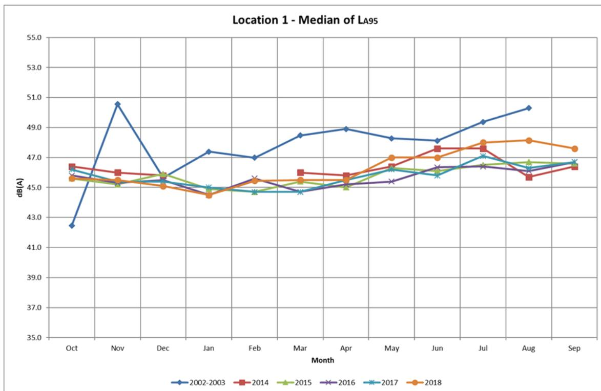
**Figure 6-2 Comparison of noise levels measured at Location 1 (North Monitor) for base period (2002 – 2003) and 2014 – 2018**
