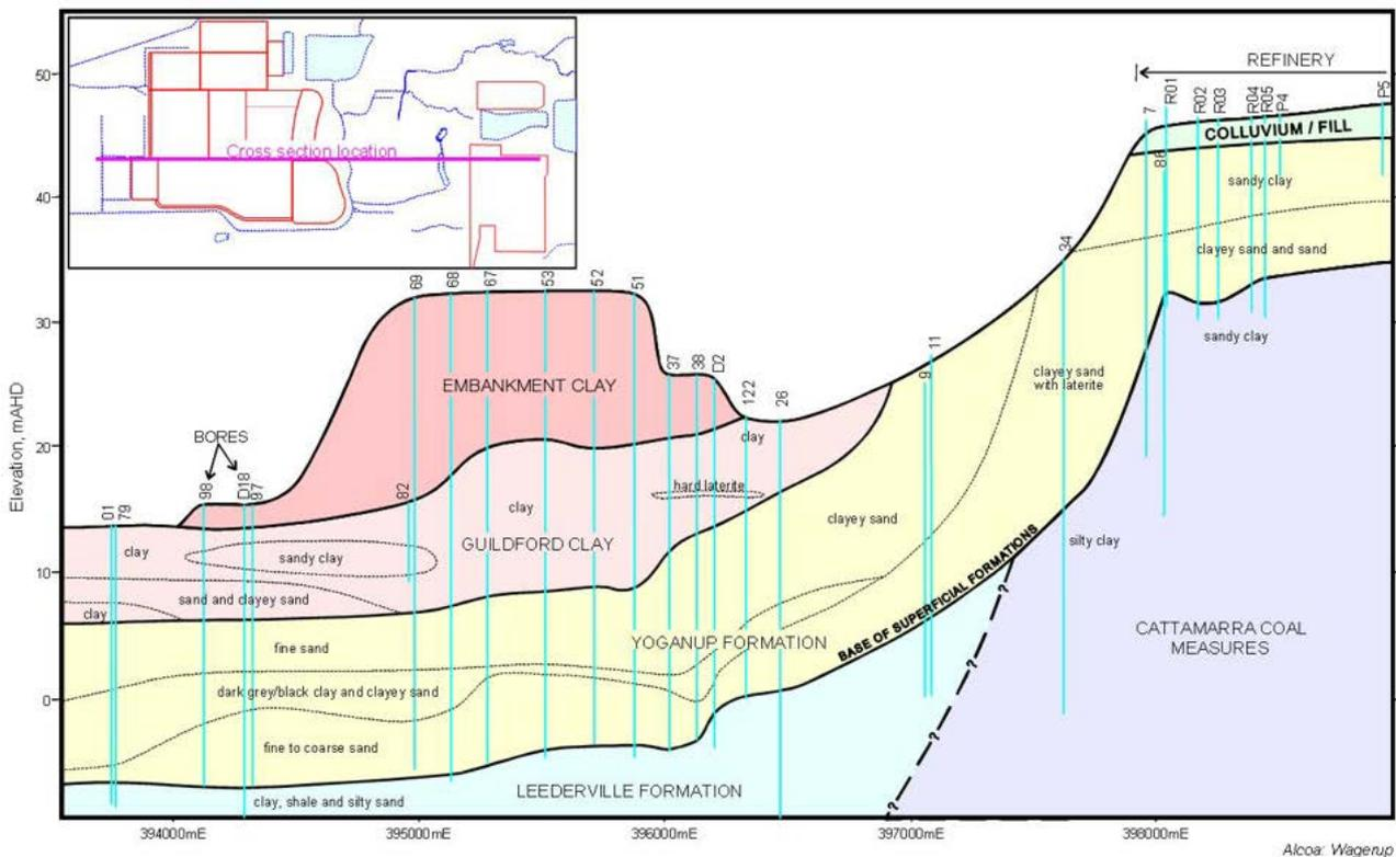
Figure 6-1: Perspective view showing schematic geological section.
