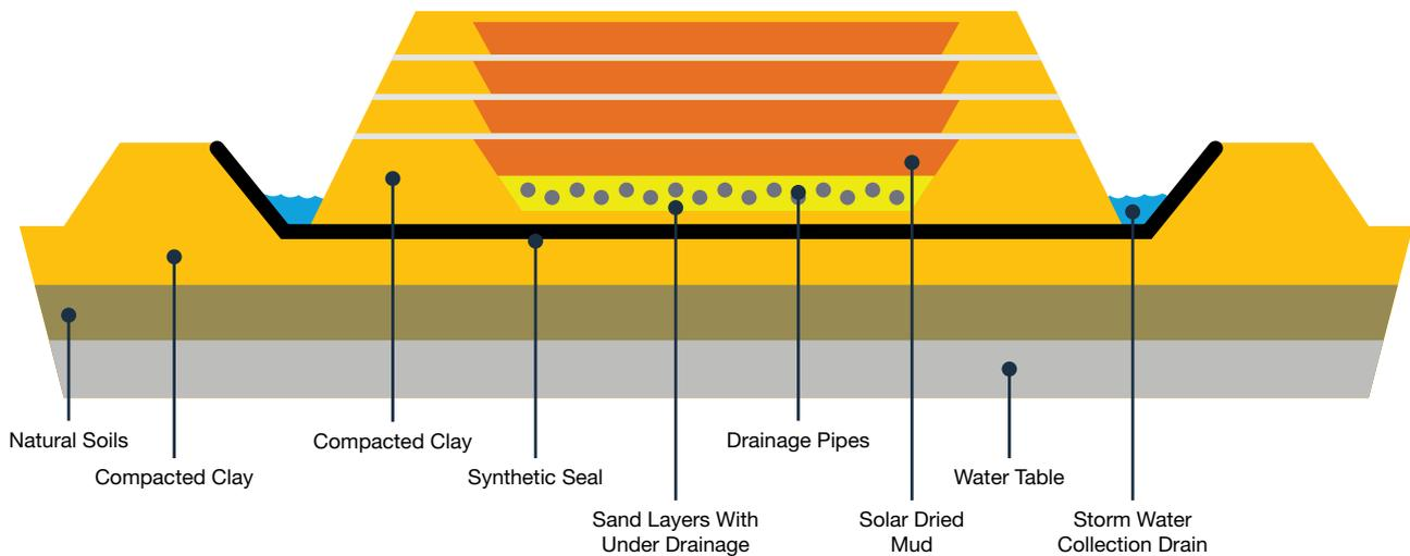
Figure 7-3: Schematic showing construction method of residue drying beds.
